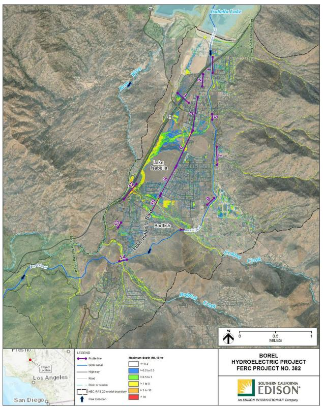
Figure 3-9. Existing Conditions Local Storm Maximum Depth – 10 Year
