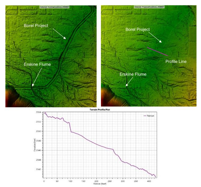
Figure 3-8. Borel Project Removal – Natural Grade Terrain
